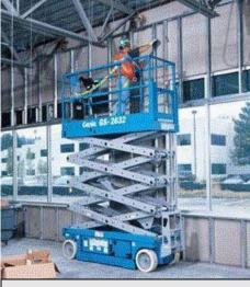
Planks, ladders or guardrail sides should not be used to gain extra reach or height. When working outside, mind the weather as wind can make a scissor lift unstable.
